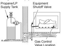
Figure 18 - Checking Gas Joints (Propane/LP Model Shown)
